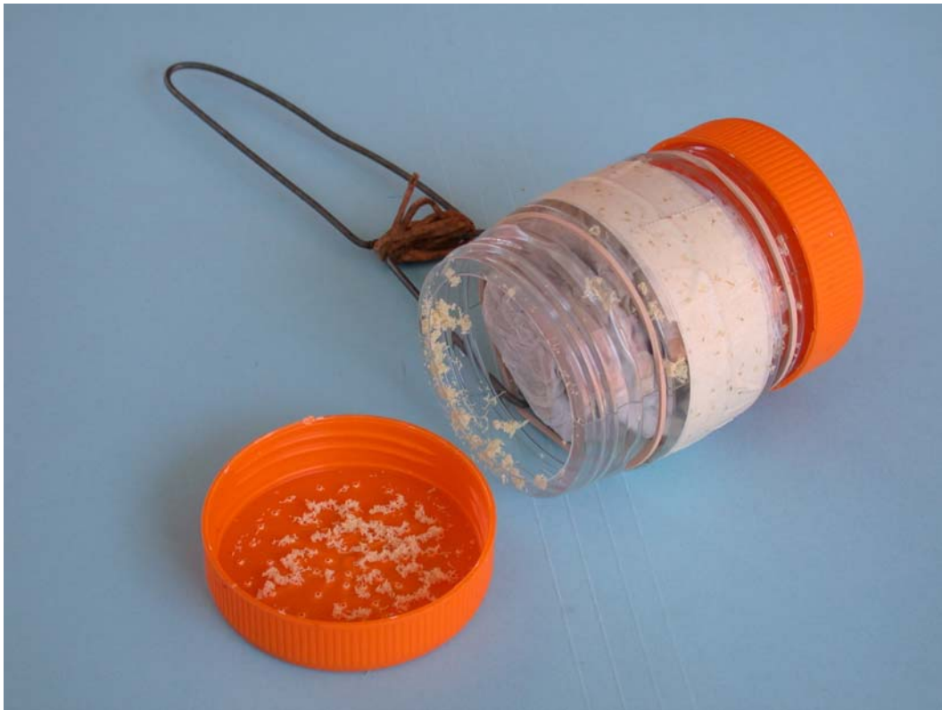
Figure 3.3.2.1.3. Egg-collection device comprising the top halves of two plastic honey jars taped together with the lids perforated with small holes to stimulate oviposition
